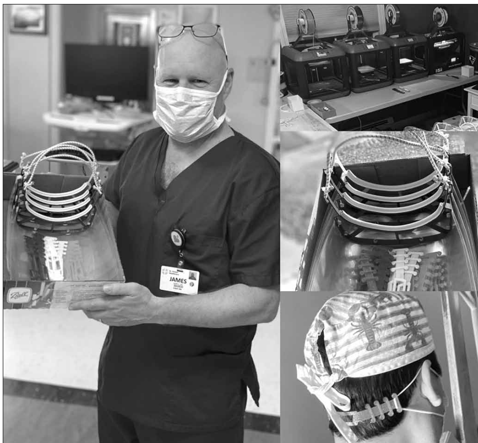
HA Technology teachers and a student used 3D printers to make face shield frames and mask backs.
